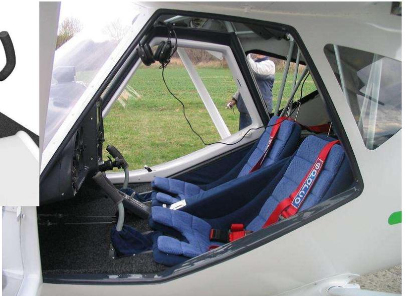
**MD-3 Rider** has all-metal semi-monocoque airframe, primary glued and riveted from aluminum alloy sheets by blind rivets.
